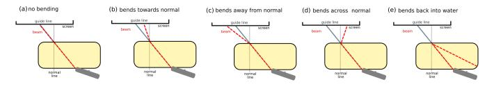
**Refraction** is the bending of a light beam when it goes from one material into another. When passing from air to water, the beam bends <u>towards</u> the normal line. When passing from water to air, it bends <u>away</u> from the normal line.
