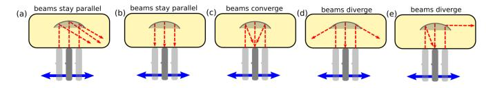
Curved mirrors change the path of incoming light beams. A **convex** mirror (curving outward) diverges the beams and a **concave** mirror (curving inward) converges the beams. When an object is reflected in the mirror, each point in the object sends of many light beams. By changing where these beams go, the mirror makes an "image" of the object --- the reflection that we see.
