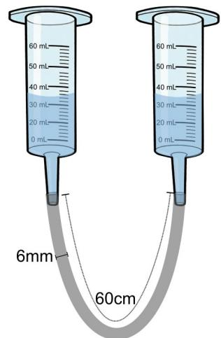
3. Now hold one syringe higher than the other, so that the 0mL mark on one lines up with the 60mL mark on the other.
