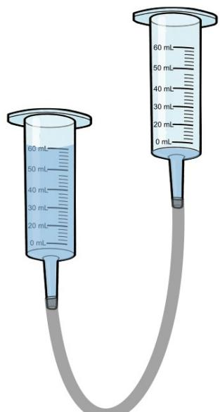
Pascal's Law states "water seeks its own level": it comes to the same height everywhere under an open surface. If one end is higher than the other, the weight of the taller column of water pushes down and makes the water move until the height is equalized.
