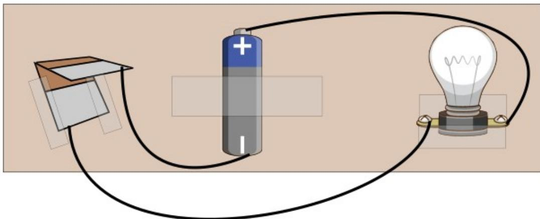
2. Attach a wire to each piece of aluminum foil, connecting it to the battery and lightbulb as shown in the diagram above. Your folded piece of cardboard is now a switch! Try pressing it down so that the aluminum pieces touch each other.
