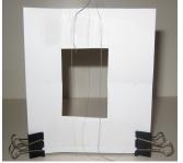
2. Shine a laser pointer at a blank screen (paper with binder clips), about 3 ft away. Place the hair in the path of the laser pointer.
